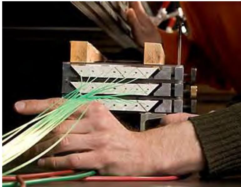
Figure 6.24: The scintillator of the P0D light yield test with the exiting WLS fibers shown.
