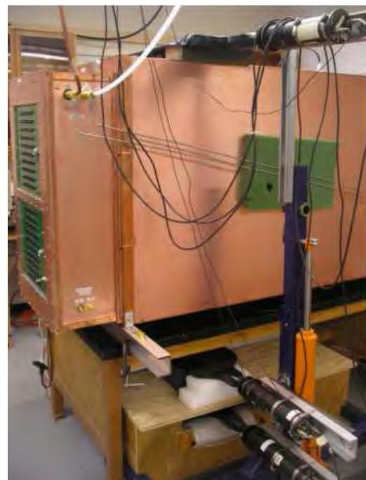
Figure 5.48: (a) The outer surface of the lower panel for the prototype. (b) the completed TPC with cosmic telescope for triggering.
