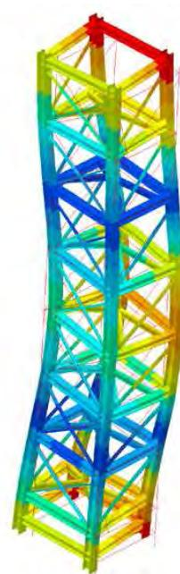
Figure 2.20: Fundamental mode of the tower
