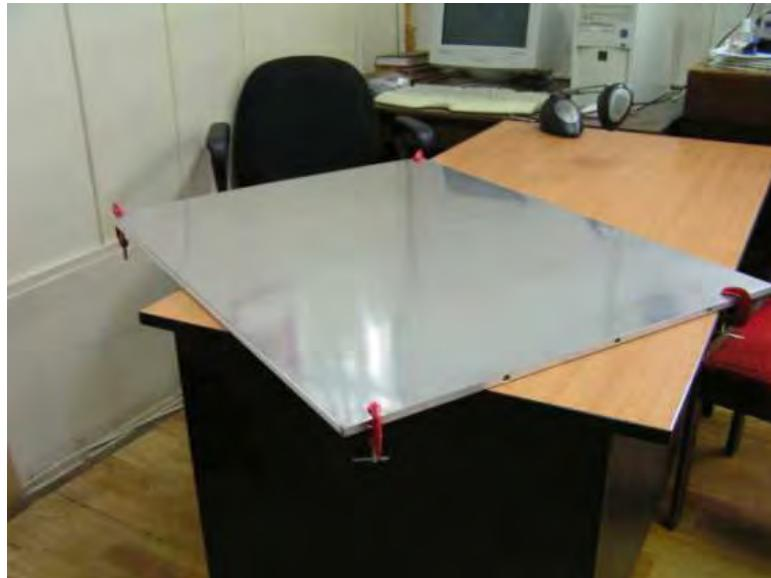
Figure 7.11: SMRD module prototype constructed at INR. 4 scintillator slabs are glued to upper and bottom stainless sheets, face sides are closed by aluminum plates with holes for optical connectors.
